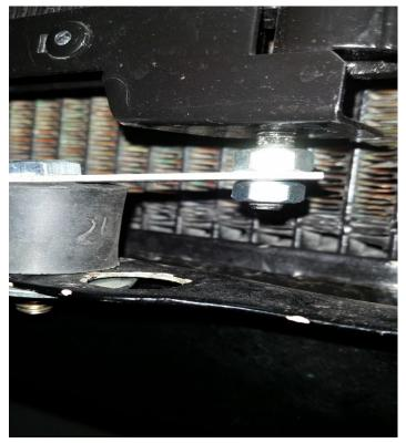
3. Bolted Compressor bracket to water pump and moved unisteer power pump back aprox. 1 inch to align pulleys and setup for belt configuration:
