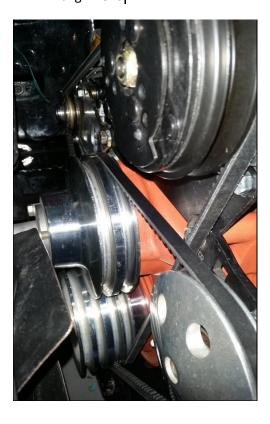
Due to Unisteer pump and non-stock billet pulleys, I had to spend some time finding the optimum belt configuration and alignment.
