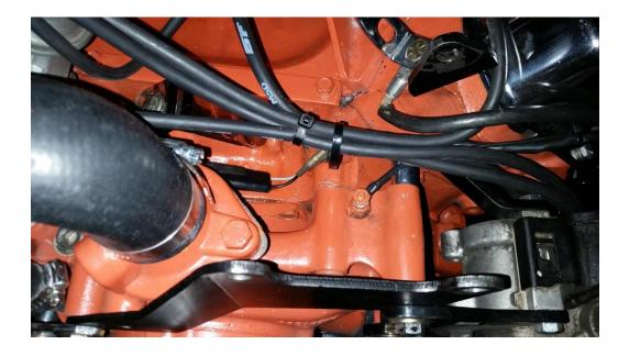
4. Modified back AC bracket to be able to move AC compressor to compensate for differences in non-OEM water pump and align pulleys:
