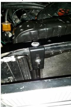
2. Bottom bracket grommets were supplied by Classic Air ( I added bracket to offset to original hole:
